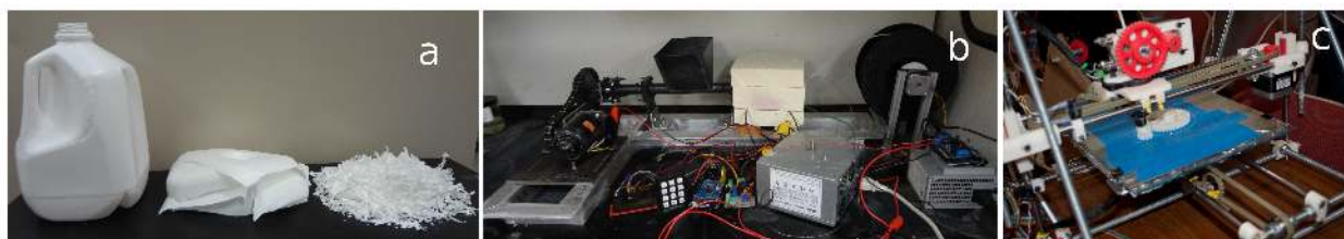
Fig. 1: Distributed HDPE Recycling. a) Cutting and shredding HDPE milk jug, b) Extruding 3-D printing filament in RecycleBot (improved performance was observed wrapping the front and back of the extruder and the insulation with Kapton tape, not shown here for clarity), c) RepRap 3-D printer self-replicating.
