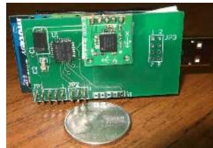
Figure 2. The sensor board with the accelerometer and gyroscope. The mother board at the back is Tmote Sky.
