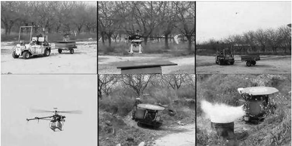
Figure 11. Some pictures of the demonstration in the ‘Alamillo’ park. The goal of the mission is to detect a fire and extinguish it with the collaboration of three robots: ROMEO-4R , HERO2 and AURIGA .
