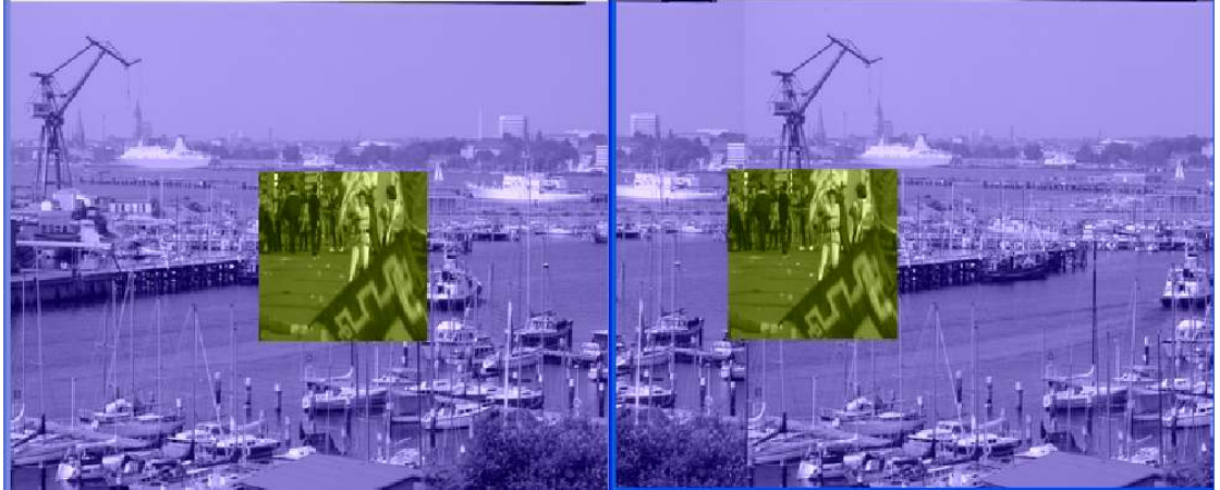
Figure 3.1.: First and last (18th) frame of the Picture-in-picture sequence. Foreground and background move opposed to each other by 5 pixels per frame.
