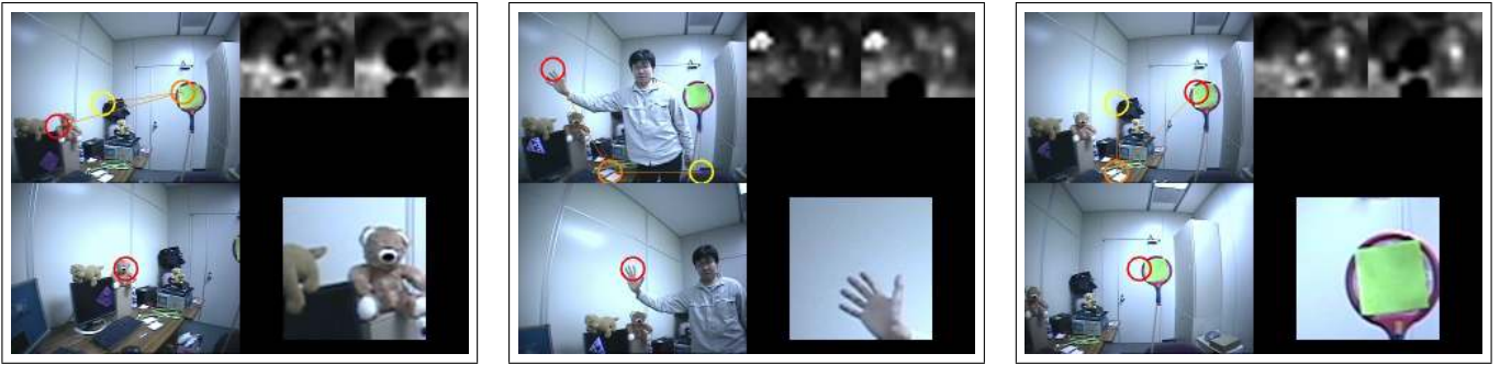
Fig. 4. Focus of attention. In each of the three images, the left upper corner shows the last image used in preattentive processing with the three last most salient locations indicated by red, orange, and yellow circle. The left lower corner shows the view from the peripheral camera after the saccade. The two smaller images in the upper right corner show the first two layers ( u_1 and u_2 ) from the system of differential equations (4) - (6). The third layer has already been reset because the images show the situation after the eyes saccaded towards the position indicated by the winner neuron. Finally, the image in the lower right corner shows the foveal view of the area of interest which could be used in postattentive processing. Note that the system detected areas that are intuitively salient.
