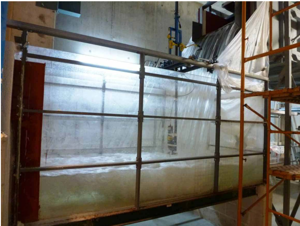
Figure 3 | Air entrainment in the plunge pool observed in the laboratory device with q = 0.082 \text{ m}^2/\text{s} , H = 2.19 \text{ m} , and Y = 0.32 \text{ m} .
