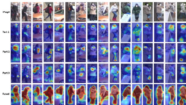
Figure 5. Visualization of the learned part-aware masks. The final mask is obtained by fusing all the part-aware masks. As we can see, these part-aware masks mainly focus on different discriminative human parts, including personal belongings.
