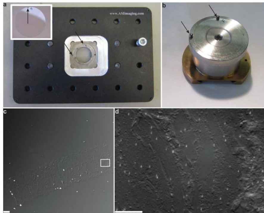
Figure 3. Tools facilitating location of the regions of interest to be imaged using different microscopy techniques. (a,b) Sample holders for fluorescent microscopy (a) and for SEM (b) that allow for precise referencing of the imaged areas. The coverslip has a notch ground using a 1/16-inch diamond bit near its top (indicated by an arrow in the inset). Both sample holders have two fixed 1/16-inch posts (indicated by arrows), which ensure unambiguous sample placement, allowing for precise coordinate referencing. (c) 10 \times DIC image of a Tokuyasu cryosection of NIH 3T3 mouse fibroblast cells used for correlative PALM and EM imaging. This can be used as a look-up map to find the area imaged in PALM when performing EM. (d) Magnified (120 \times ) DIC image of the area in the rectangle in c, imaged during the PALM step. Scale bars, 40 \mu m (c); 10 \mu m (d).
