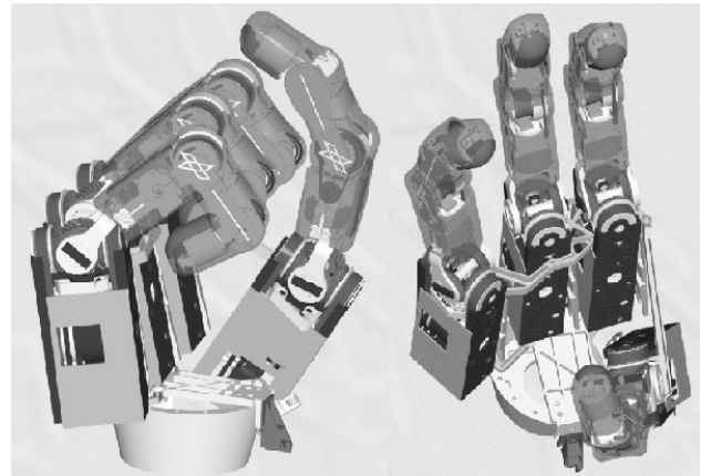
Figure 4. Simulation of Hand II in power-grasp- and fine manipulation configuration.
