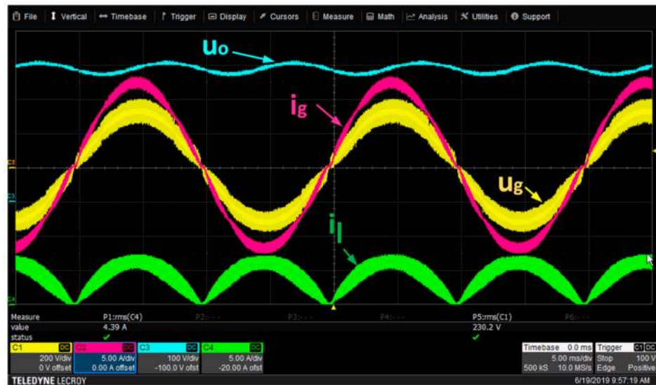
Figure 14. Measured waveforms of two units interleaved using parameters ( f_{sw} = 20 kHz) and a phase shift of 180^\circ given in Table 5.
