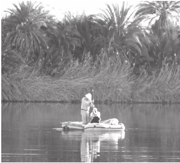
Figure 4. Coring Lake Gabr 'Awn using a Livingstone piston corer system from boats moored in the lake.
