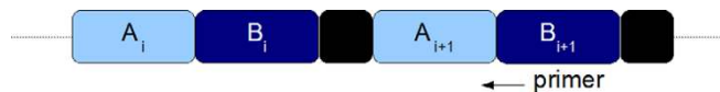
Figure 1 DNA One-Time pad. A_i : plain text, B_i : cipher text (and primer for the DNA polymerase), black box: stop Modified from Gehani et al. [2].
