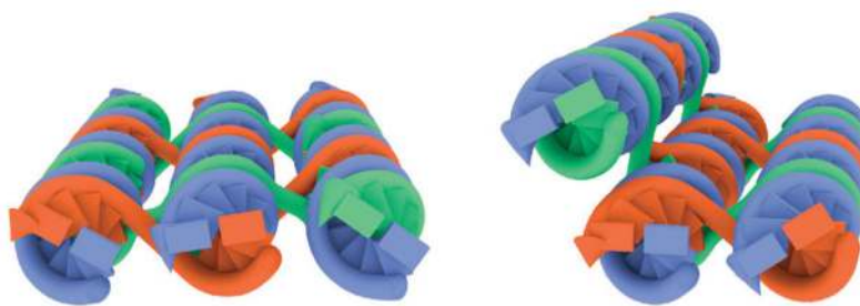
Fig. 2. Distances between crossovers define the angle between helices. Left: an integer number of half turns results in a 2D structure. Right: a non-integer number of half turns results in a 3 dimensional structure. In this case an angle of 120^\circ is achieved by a 7 base pair distance between crossovers.
