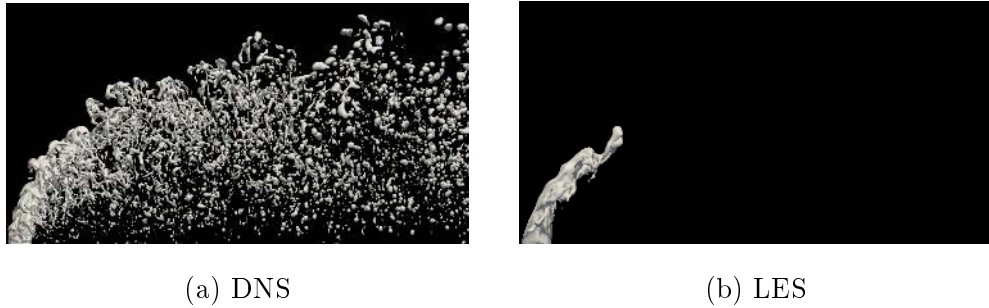
Figure 1: Instantaneous snapshots of the side view of the atomizing liquid jet obtained from DNS and LES.
