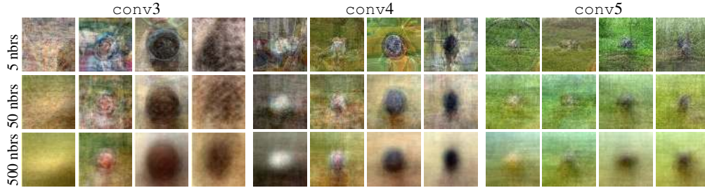
Figure 2: Similar convnet features tend to have similar receptive field centers. Starting from a randomly selected seed patch occupying one rf in conv3 , 4, or 5, we find the nearest k neighbor features computed on a database of natural images, and average together the corresponding receptive fields. The contrast of each image has been expanded after averaging. (Note that since each layer is computed with a stride of 16, there is an upper bound on the quality of alignment that can be witnessed here.)
