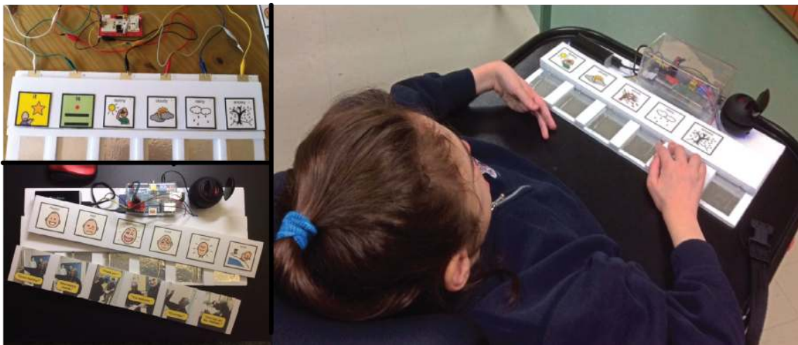
Figure 1. The first prototype (top left) consists of a computer (not shown) and a Makey Makey board connected to a hand-made foam board fitted with aluminum foil touch-switches and labeled with replaceable printed symbols. TalkBox (bottom left and in use, right) consists of a Raspberry Pi connected to a capacitive touch sensor, speakers and a hand-made foam board with aluminum foil touch switches
