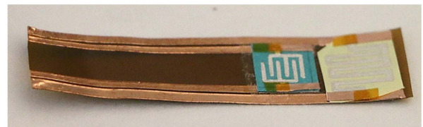
Fig. 1. Sticker with paper based humidity and temperature sensor attached using anisotropic conductive tape DIY integration approach
