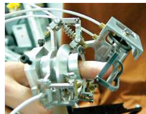
Figure 3: Location display that operates by rolling a servo-controlled plate on the fingertip as a function of the exploratory movements of the finger [27].
