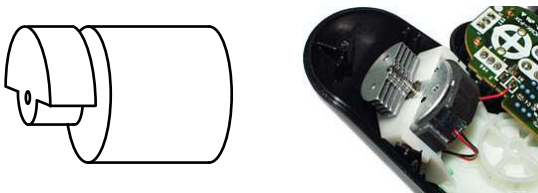
Figure 4: The rumble motor. An eccentric mass spun by a DC motor.
