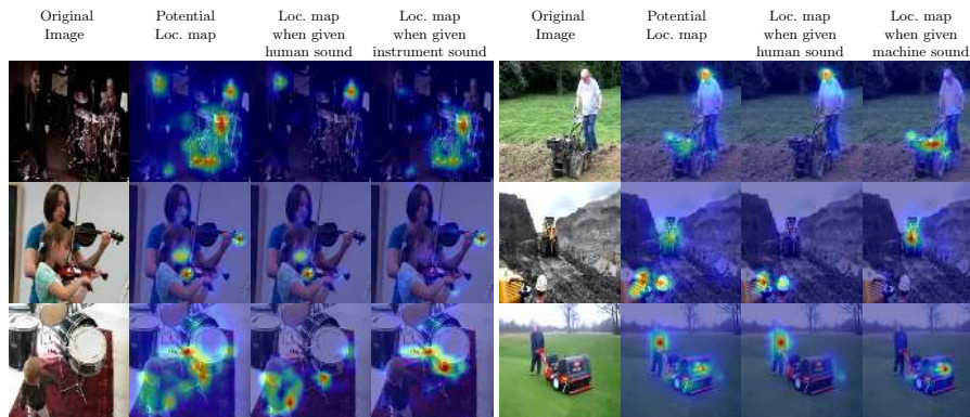
Fig. 5. Visualization results of potential localization maps and localization maps of samples with several objects capable of producing sound in the image, but of which only one object is actually producing sound (Type B). The localization map successfully responds to an object that is actually producing sound, while the potential localization map does not. For the visualization, we use the model trained with 144k samples and pretrained weights.
