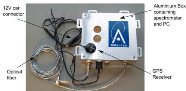
Fig. 2. The ULM-DOAS instrument. Inside the box are a compact UV-Vis spectrometer and a PC-104. Light is collected directly by the optical fiber and a GPS is used to geolocalize the measurements. The whole system is powered with 12 V.
