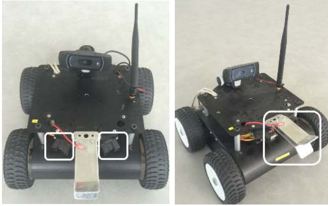
(a) IRs distance sensors (b) Dock connector
