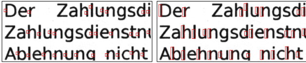
Fig. 3. A comparison of the fixed size windows (left) and dynamic height windows (right) approach. The red boxes mark the detected edges which serve as the basis for the feature extraction.
