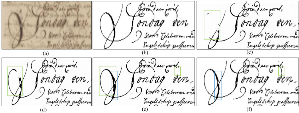
FIGURE 13. Binarization results from the different configurations (a) original image, (b) the ground truth, (c) Baseline, (d) Baseline + stroke boundary feature extracting module, (e) Baseline + stroke boundary feature extracting module + feature fusion module, (f) Baseline + stroke boundary feature extracting module + feature fusion module + discriminator (our proposed method). Green boxes aim to compare in connected stroke level. Blue boxes compare in sharp stroke level.
