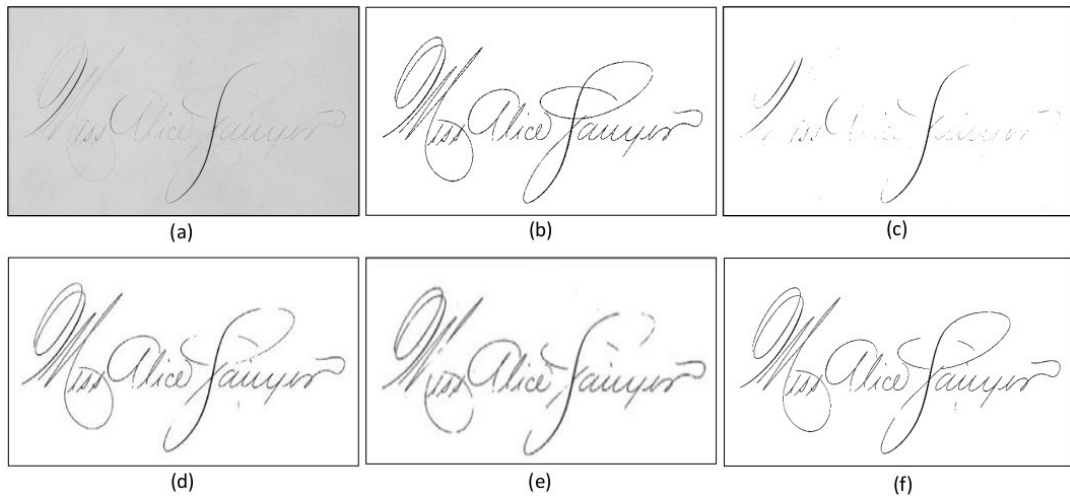
FIGURE 9. Results of binarization methods on the degraded document image with the long and thin strokes (sample HP6 in DIBCO 2013). (a) Shows the degraded document image. (b) Is ground-truth. (c) Is the result of Otsu method [9]. (d) Displays the result of DSN [6]. (e) Is the result of cGANs [5]. Our proposed method is illustrated in (f).
