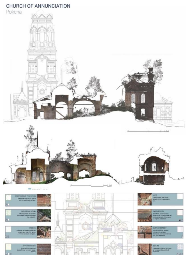
Figure 6. Point cloud views and drawings with analysis of the decay of the Church of Annunciation.
