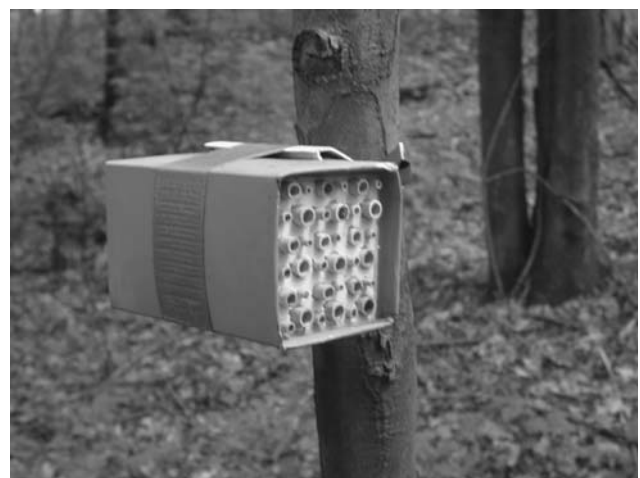
Fig. 1 Nest box constructed from a 2-l milk carton ( 9.5 \times 9.5 \times 16.5 cm 3 ) with a polystyrene piece. Each box contained 36 cardboard trap-tubes; nine of each 3, 5, 7 and 9 mm internal diameters \times 15 cm length
