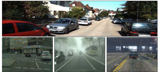
Figure 1. Illustration of different datasets for autonomous driving: From top to bottom-right, example images are taken from: KITTI[17], Cityscapes[5], Foggy Cityscapes[49], SIM10K[30]. Though all datasets cover urban scenes, images in those dataset vary in style, resolution, illumination, object size, etc. The visual difference between those datasets presents a challenge for applying an object detection model learned from one domain to another domain.
