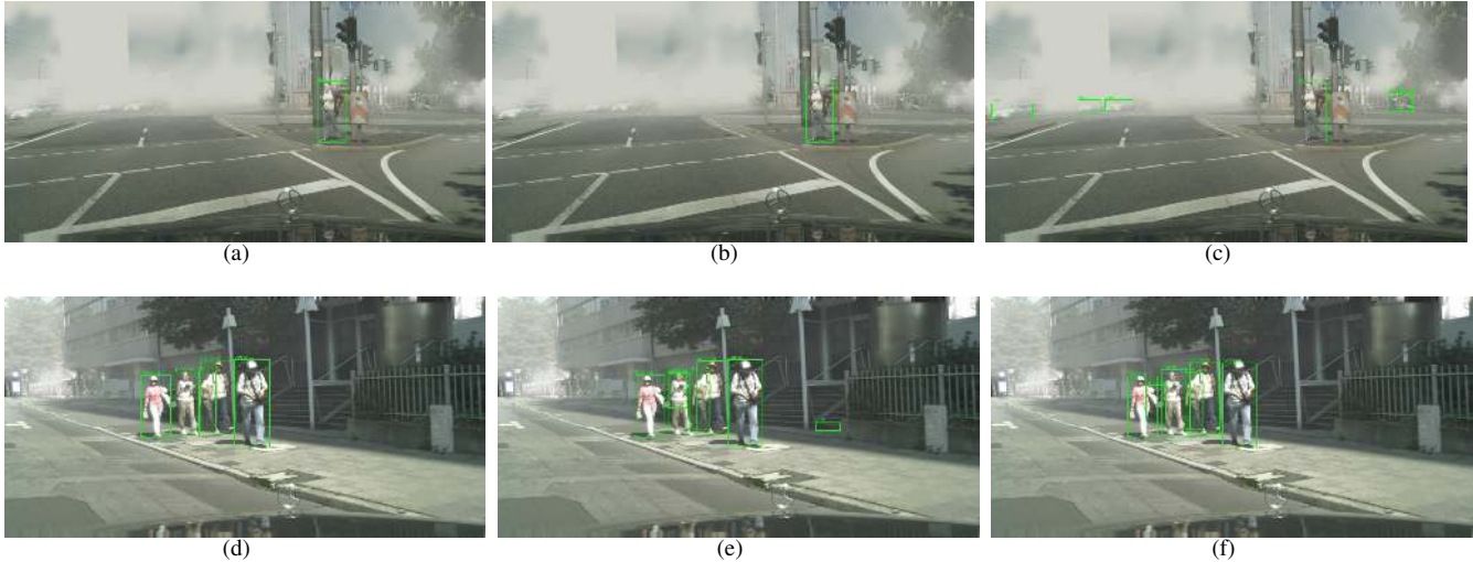
Figure 6. Object Detection Display Fig 6(a)-6(c) and 6(d)-6(f) present two set of detection results on different inputs. Results from left to rights each line are detected by source-only Faster R-CNN, UDA framework and UDA framework with DSS respectively.
