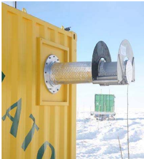
Figure 5: The Pre-HEAT telescope installed onto the PLATO instrument module at Dome A. Photo from January 2008, courtesy Z. Zhu and Z. Xu.
