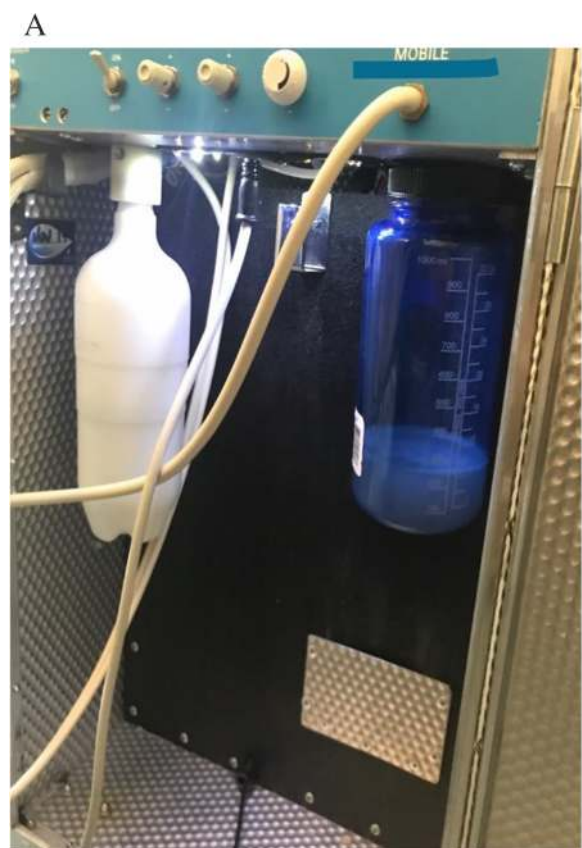
Main case for the compressor, water tanks, handpieces and suction. This case weighs approximately 17 kg
