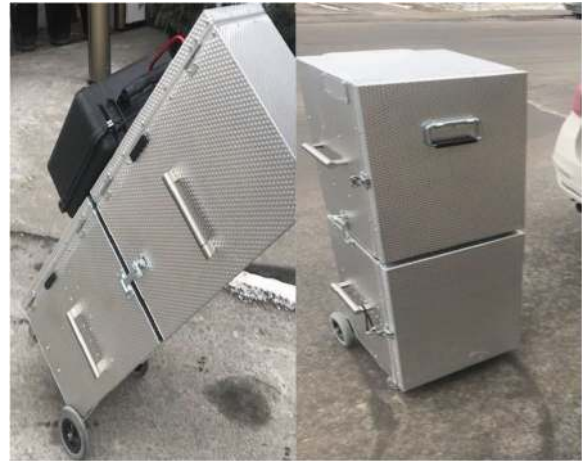
This unit is composed of two stackable aluminum cases. The dimensions of the stacked cases are 13"x 51" x 16".
