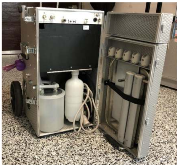
The aluminum case contains the compressor and the clean/used water tanks linked to the handpieces and suction, as well as a movable tray.
