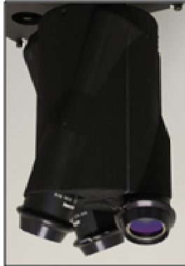
Figure 4. Prototype Doppler lidar system consisting of an electronic chassis and an optical head. All the lidar components, including transmitter laser, photoreceivers, and real-time processor, are housed in the electronic chassis. The optical head consists of three transmit and receive lenses connected to the electronic chassis by a fiber optic cable.
