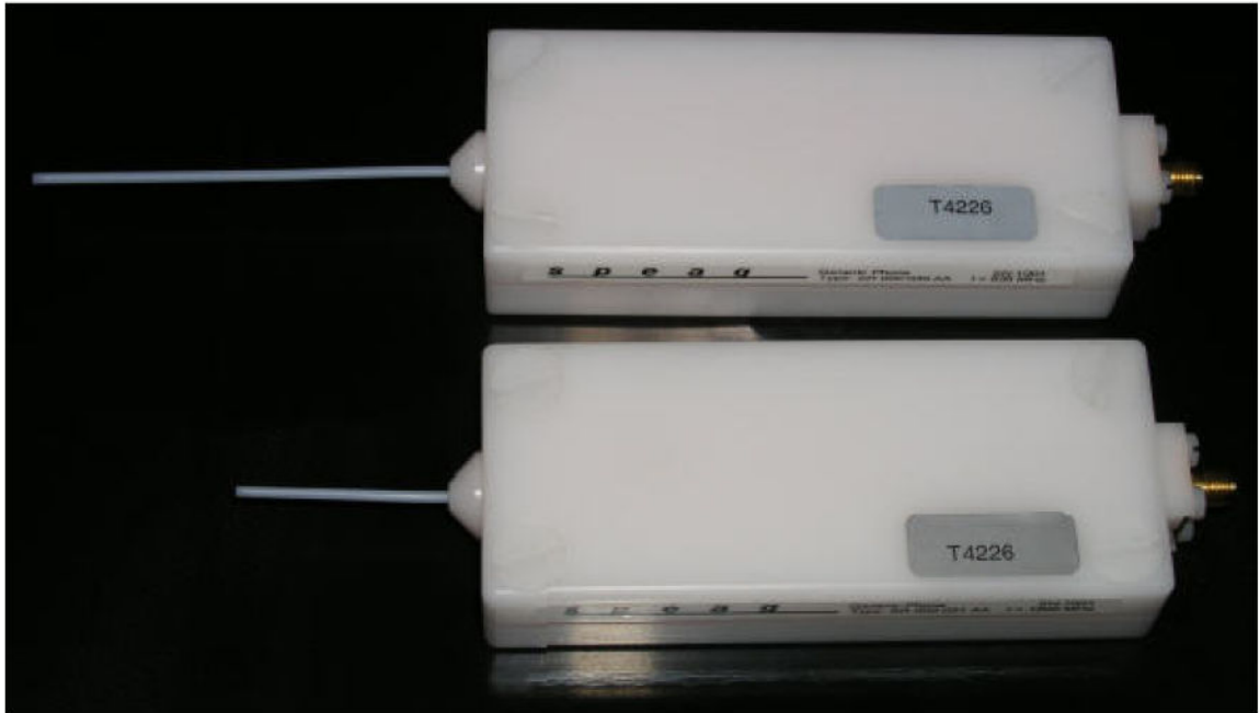
Figure 15. Generic phones for the measurement on the SAM phantom. The upper picture shows the phone for 835 MHz, the lower for 1900 MHz.
