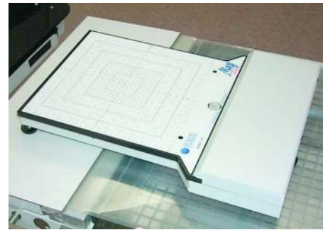
FIG. 2. Example of a matrix detector.
