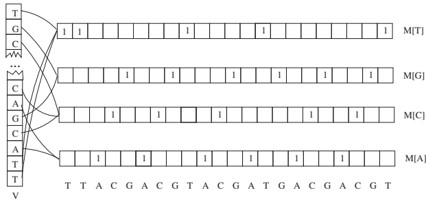
Fig. 1. Sample data structure for the matrix associated to the sequence TTACGACGTACGATGACGACGT
