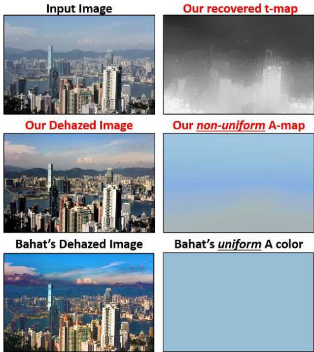
Figure 10: Uniform vs. Non-Uniform Airlight recovery. The uniform airlight assumption is often violated (e.g., in dusk and dawn). Double-DIP allows to recover a non-uniform airlight map, yielding higher-quality dehazing.
