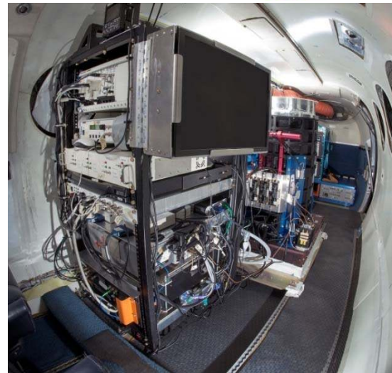
2- \mu double-pulse IPDA lidar
