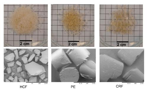
**Figure 3.** Photograph (**top**) and SEM micrograph (**bottom**) of different feedstocks for milling. From left to right: HCF, PE, CRF.
