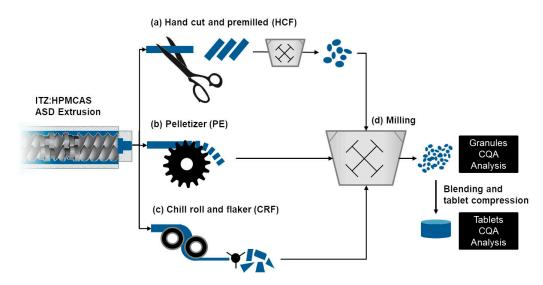
**Figure 1.** Downstream processing of extruded strands by hand-cutting (**a**), pelletizing (**b**), and chill roll technology (**c**) and subsequent milling (**d**).
