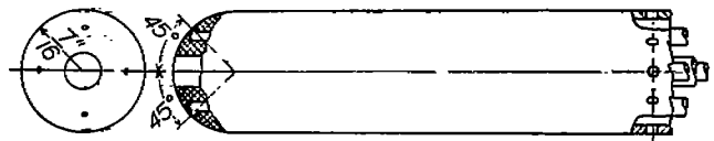
FIGURE 2.—Line drawing showing combined pitch, yaw, and pitot-static tube used for the dynamic-pressure and the downwash surveys.
