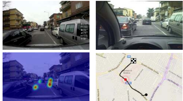
Figure 1. An exemplar frame from our dataset. From left to right, from up to bottom: car-mounted view, driver's point of view, gaze map overlay and geo-referenced course.
