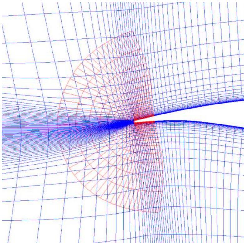
Figure 12. DLR-F6 WB Volume Grid at Wing Trailing-Edge.
