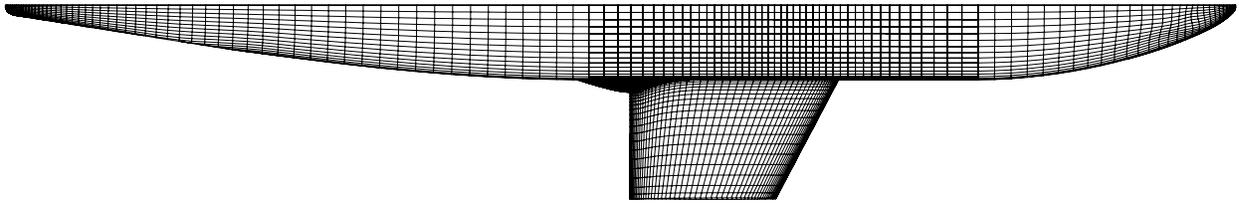
Figure 5. Top View of Baseline DLR-F6 Fuselage with FX2 WB Fairing.
