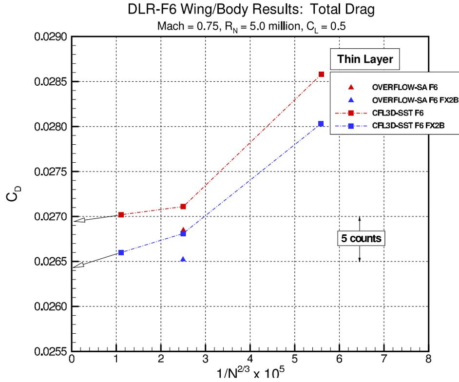
Figure 23. DLR-F6 Grid Convergence Study: Thin-Layer Total Drag.
