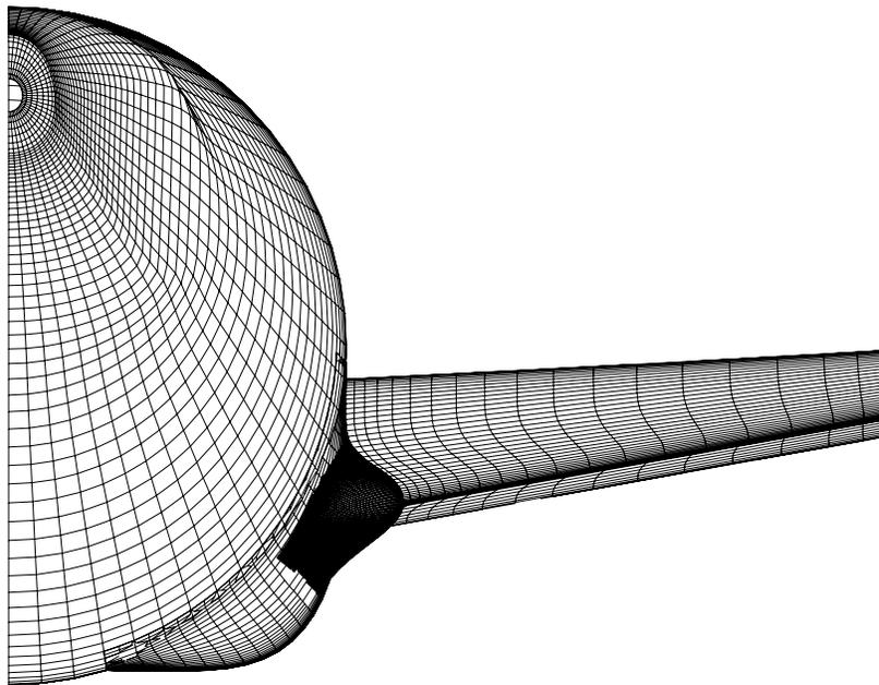
**Figure 4. Rear View of Baseline DLR-F6 Fuselage with FX2 WB Fairing.**
