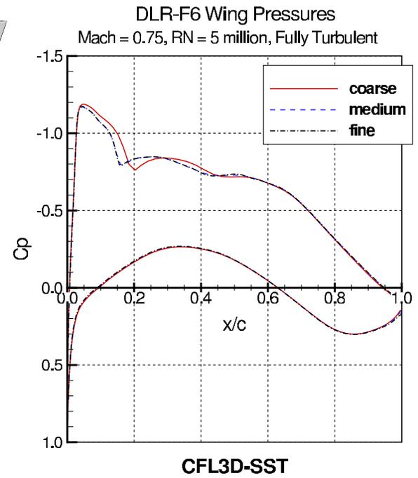
Figure 26. DLR-F6 Wing Pressure Comparison at .637 Semispan.
