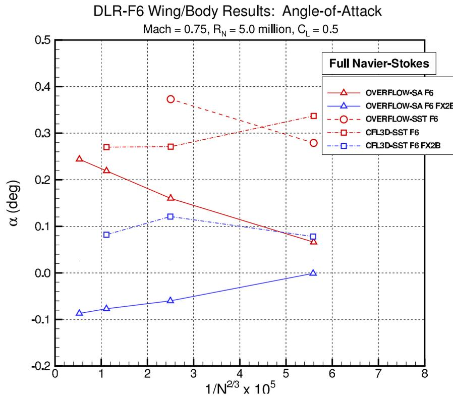
Figure 20. DLR-F6 Grid Convergence Study: Full Navier-Stokes Angle-of-Attack.
