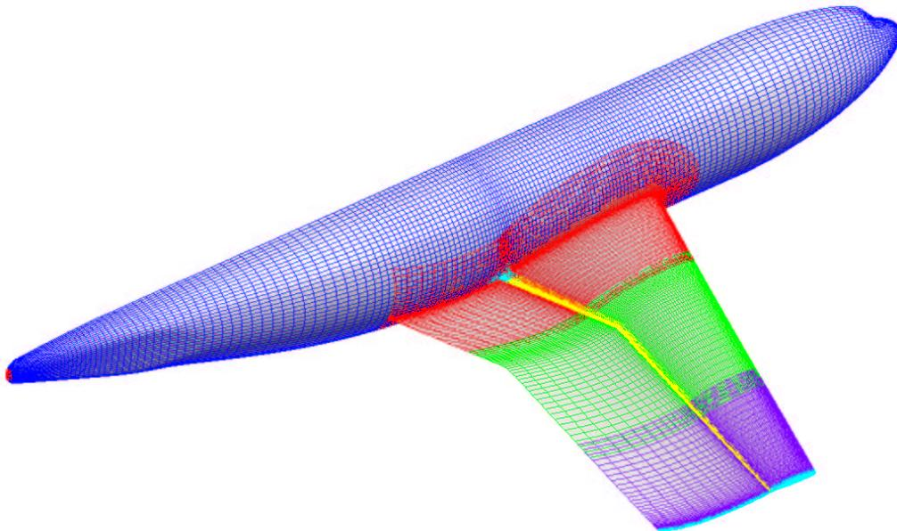
Figure 6. DLR-F6 WB Overset Surface Grids.
