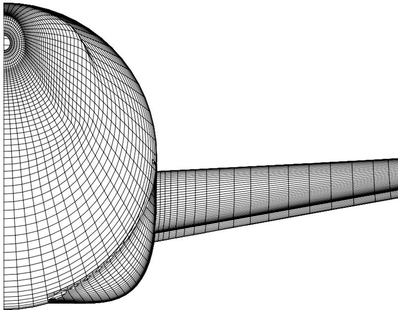
**Figure 3. Rear View of Baseline DLR-F6 Fuselage with FX1 WB Fairing.**
