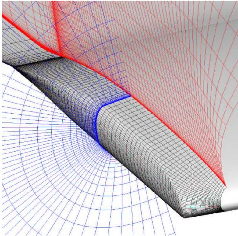
Figure 11. DLR-F6 WB Volume Grid at Wing Tip.
