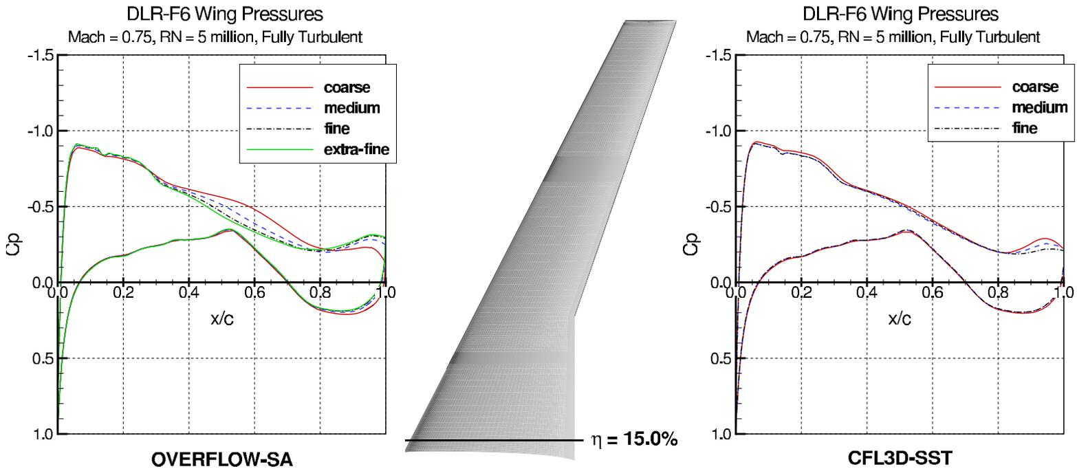
Figure 24. DLR-F6 Wing Pressure Comparison at .150 Semispan.
