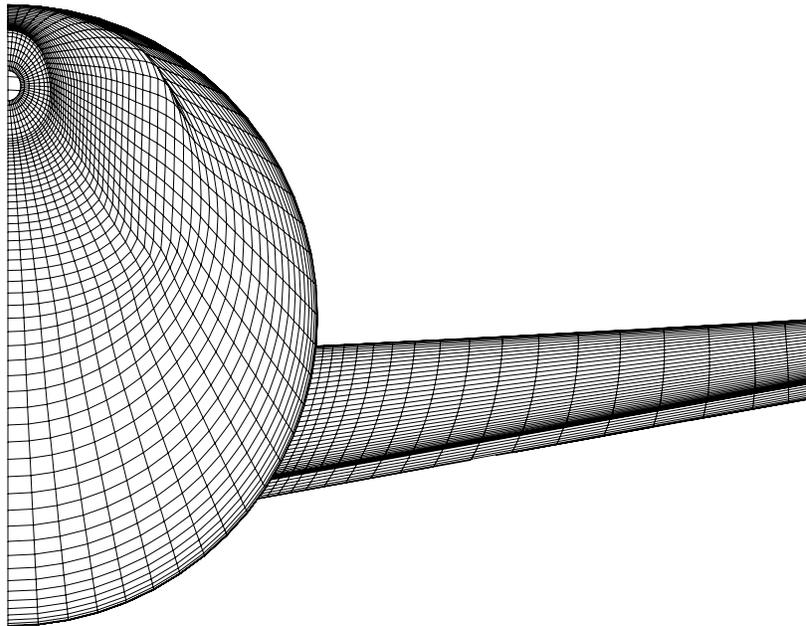
Figure 2. Rear View of Baseline DLR-F6 Fuselage and Wing Root.
