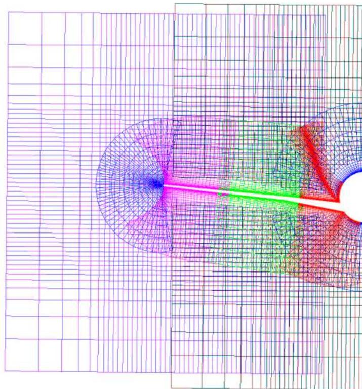
Figure 10. DLR-F6 WB Volume Grid at Wing Mid-Chord.
