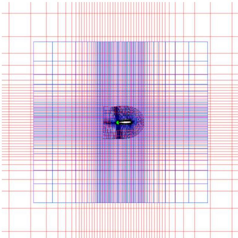
Figure 14. DPW-W1/W2 Volume Grid at Symmetry Plane.
