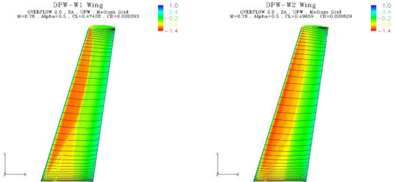
Figure 49. DPW-W1/W2 Surface Streamline Comparison at  $\alpha = 0.5^\circ$ .
