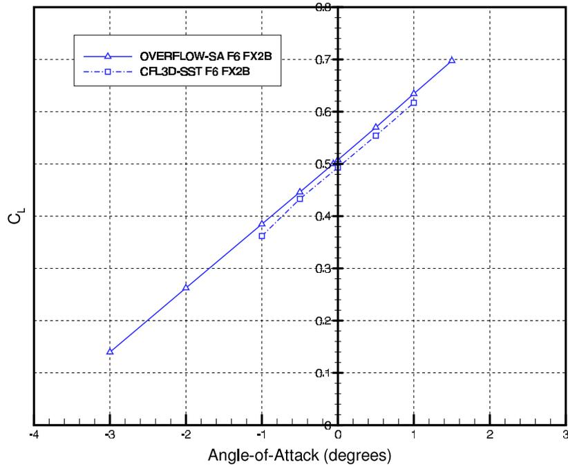
Figure 33. DLR-F6 Lift Curve: F6 FX2B.
