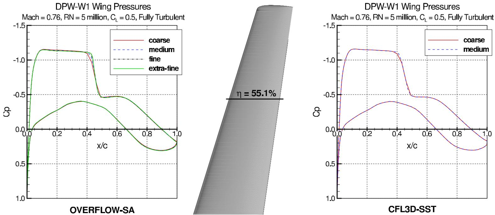
Figure 45. DPW-W1 Wing Pressure Comparison at .551 Semispan.
