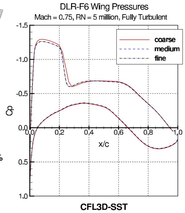
Figure 25. DLR-F6 Wing Pressure Comparison at .332 Semispan.
