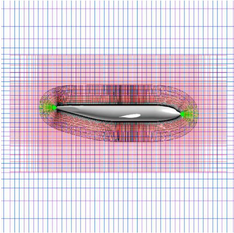
Figure 7. DLR-F6 WB Volume Grid at Symmetry Plane.
