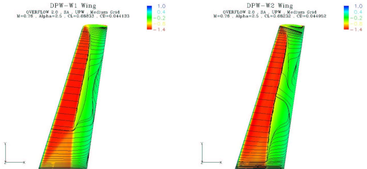
Figure 51. DPW-W1/W2 Surface Streamline Comparison at  $\alpha = 2.5^\circ$ .
