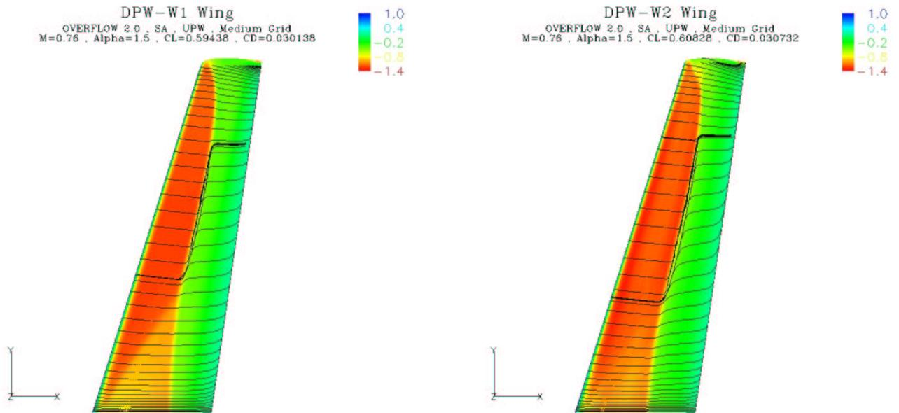
Figure 50. DPW-W1/W2 Surface Streamline Comparison at  $\alpha = 1.5^\circ$ .
