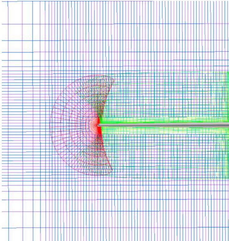
Figure 15. DPW-W1/W2 Volume Grid at Wing Mid-Chord.
