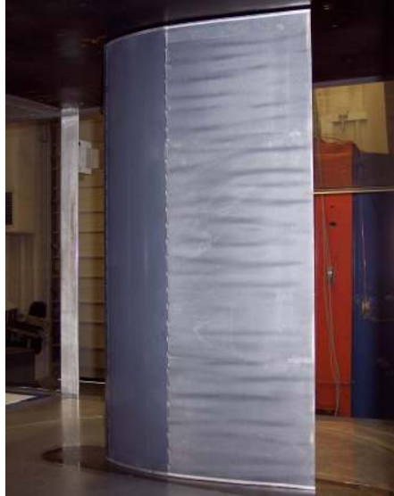
Figure 3. DU 96-W-180 model in the wind tunnel with riblet film on the upper surface turbulent region.
