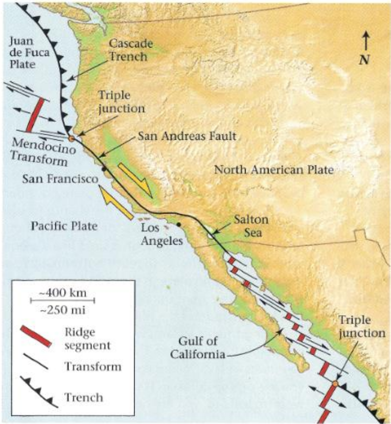
Figure 4 the west coast of the United States (oblique view) showing the triple junction(MTJ) where the Cascade trench, the Mendocino Transform and the San Andreas Fault meet (Marshak, 2001).
