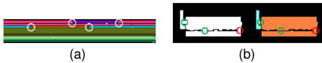
Fig. 24. (a) The narrow regions are over-segmented due to noisy points. The white circles mark the over-segmented edges. (b) The red-circled gap is failed to be closed and the green-circled gaps are closed well.
