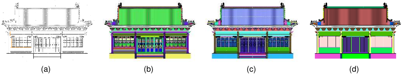
Fig. 3. The drawing segmentation procedure. Every group is colored differently for distinction. (a) The input drawing with user-drawn orange segments used to prevent over-aggressive grouping. (b) The drawing is first segmented into region groups. (c) The region groups with compatible repetitive patterns are clustered to vote for repetitive patterns. The region groups in the same equivalence classes are painted in the same color and the pattern centers are painted with white circles. (d) Finally, based on the repetitive patterns, the region groups are clustered to form meaningful component groups.
