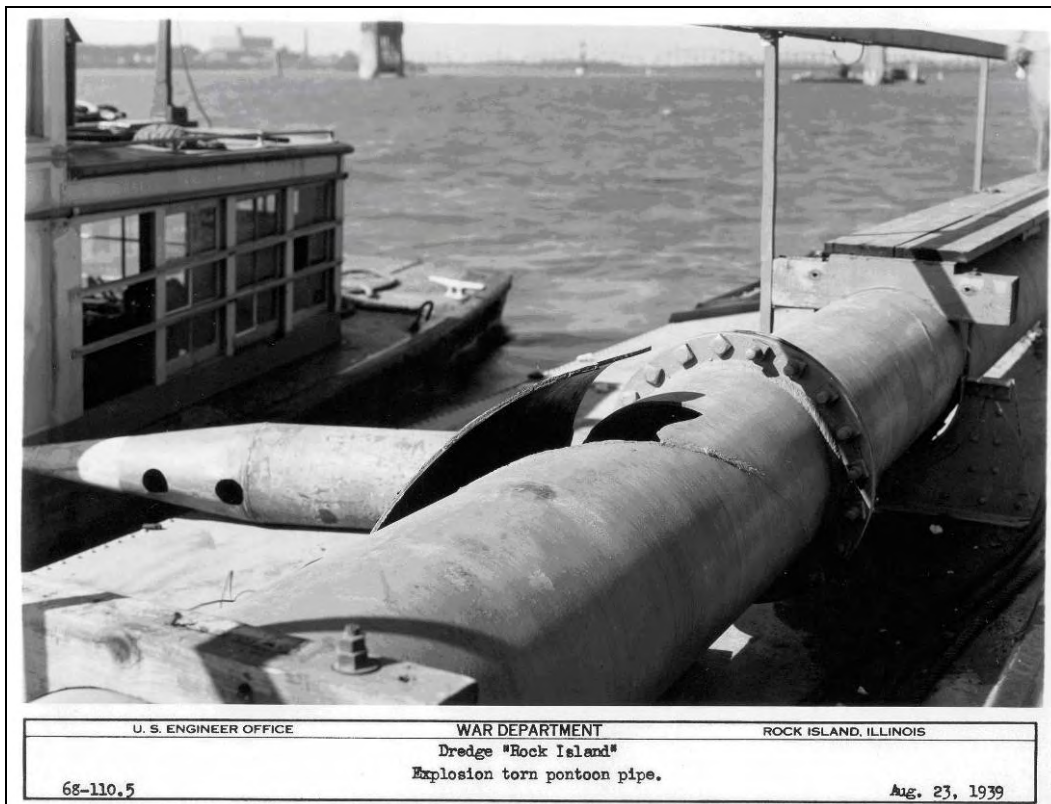
Figure 47. Explosion-torn pontoon pipe of dredge Rock Island (courtesy of Rock Island District).
