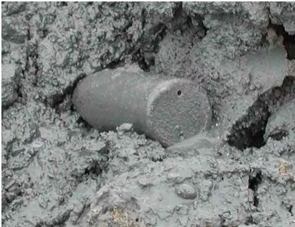
Figure 80. A 5 in. brass training round; first DMM discovered in Baltimore Harbor dredging project.
