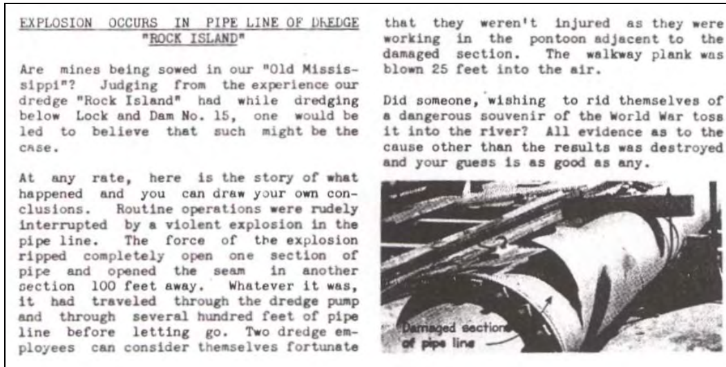
Figure 46. Hydraulic cutterhead pipeline dredge encounter with UXO excerpt from Rock Island District's publication The Safe Channel , September 1939 (courtesy of Rock Island District).
