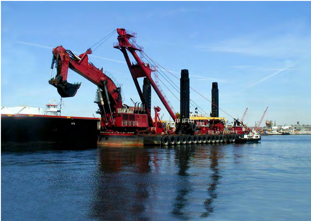
Figure 2. Backhoe dredge New York (courtesy of Great Lakes Dredge and Dock Company).
