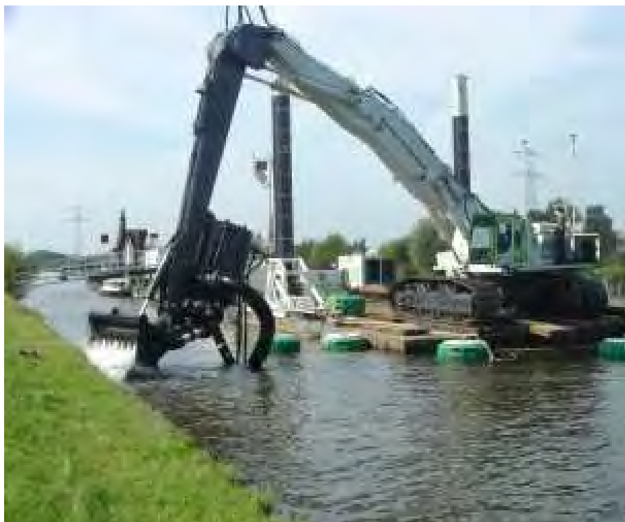
Figure 23. Backhoe-mounted submersible pump with MEC-exclusion screen and activated jet water system (courtesy of Damen Dredging Equipment, The Netherlands).
