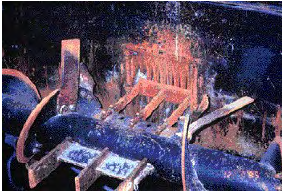
Figure 69. Front view of augerhead suction mouth screen/cutter device (source: Walsh and Collins 1998).
