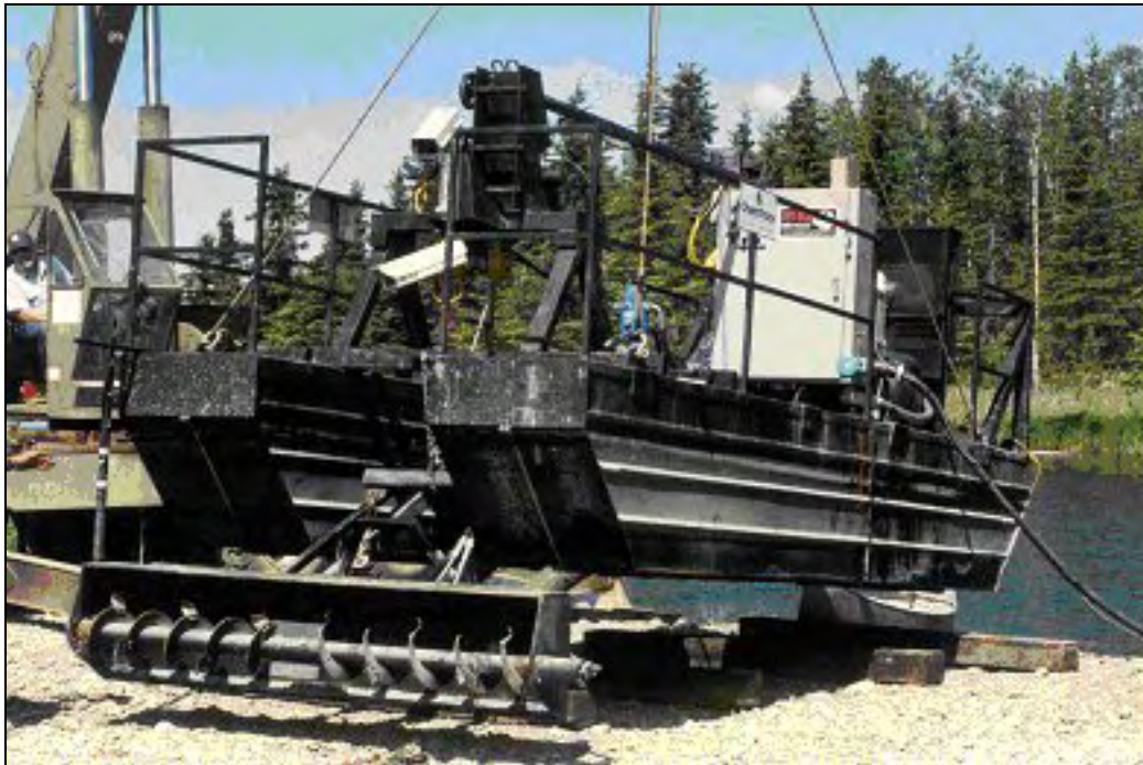
Figure 61. The PITHOG electric remote control lagoon pumper.
