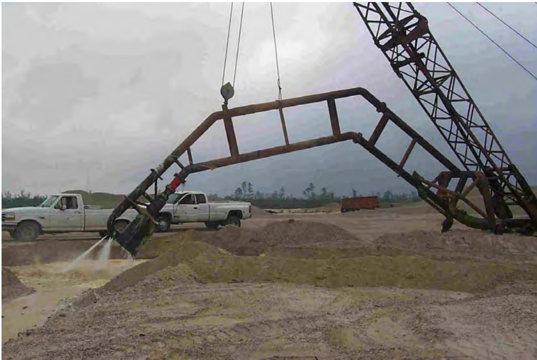
Figure 13. Standard Gravel Company (Genflo) eductor used in MEC trial.
