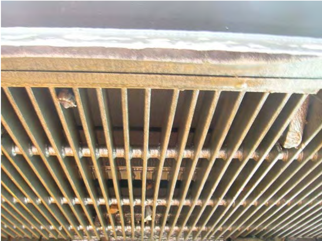
Figure 37. Draghead screen on hopper dredge R.N. Weeks at Bethany Beach, DE (2007). Apertures sized to 32 mm × 292 mm (source: Weeks Marine Inc.).
