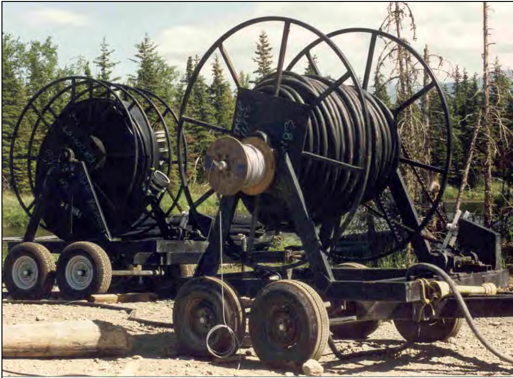
Figure 64. Flexible discharge hose and power cable on mobile spools.
