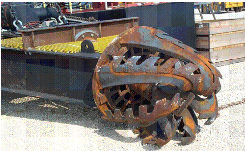
Figure 58. Gatling Gun suction screen installed on cutterhead (source: DSC).
