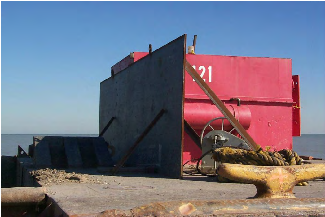
Figure 113. Scow release operator's protective barrier.
