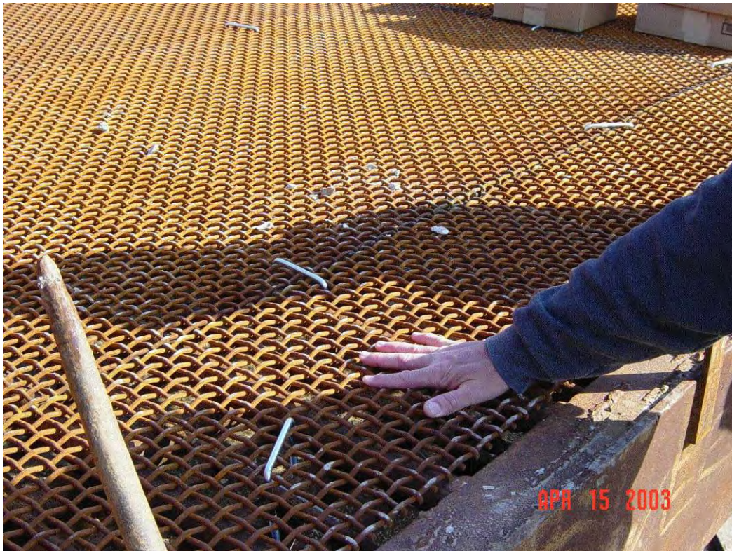
Figure 86. Static screen with approximately 25.4 mm (1 in.) square apertures used at HMI.
