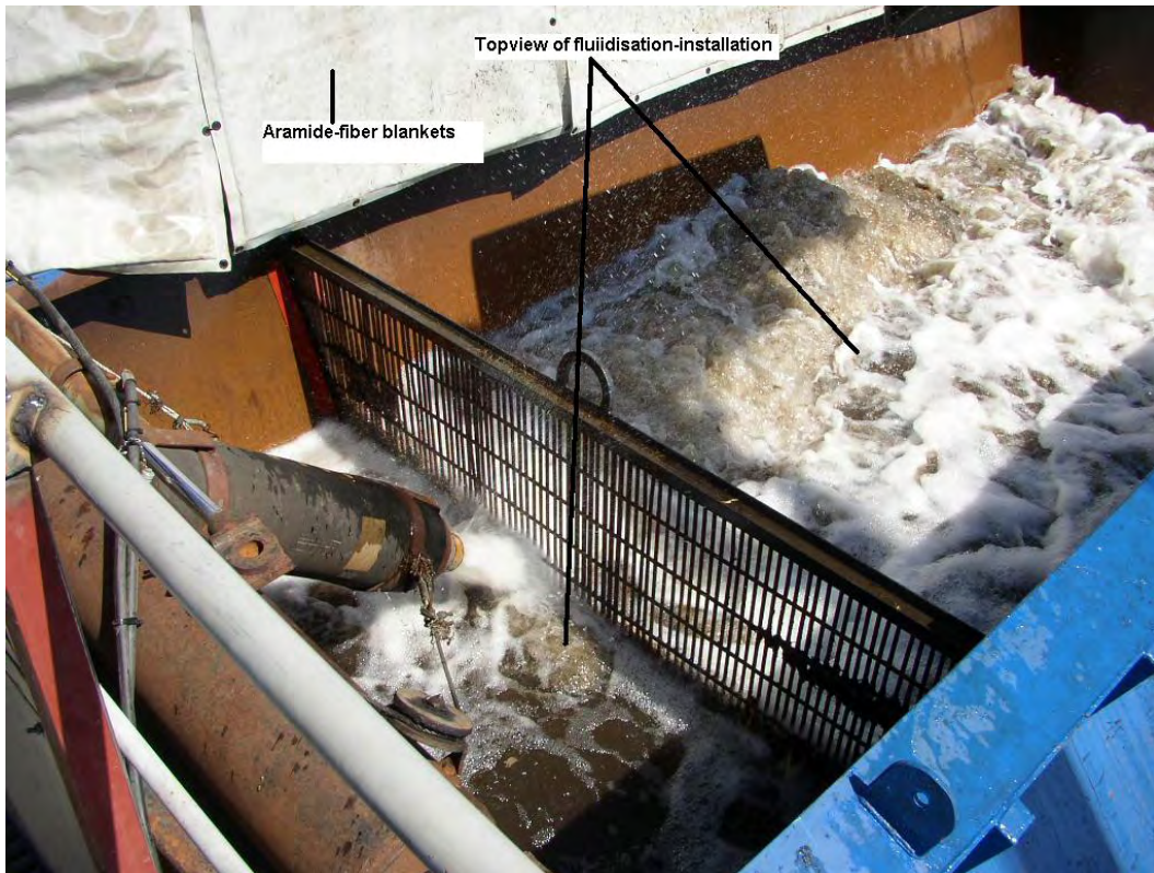
Figure 93. Waterjet applied to MEC-contaminated sediment (courtesy of Heuvelman Ibis BV).
