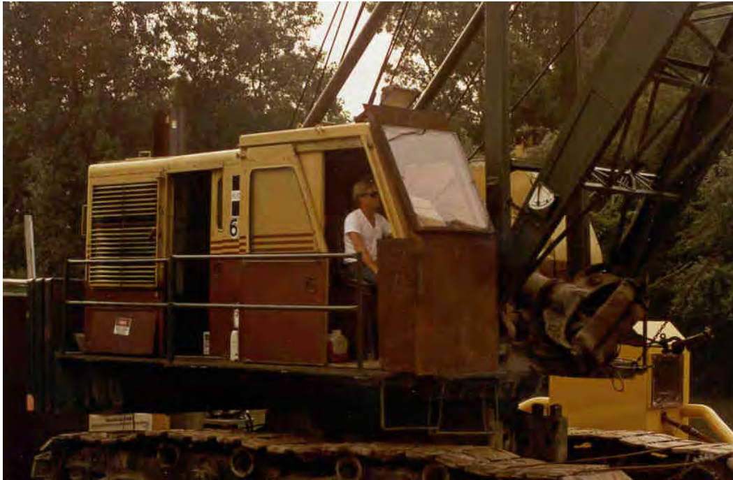
Figure 97. Crane operators protective barrier.
