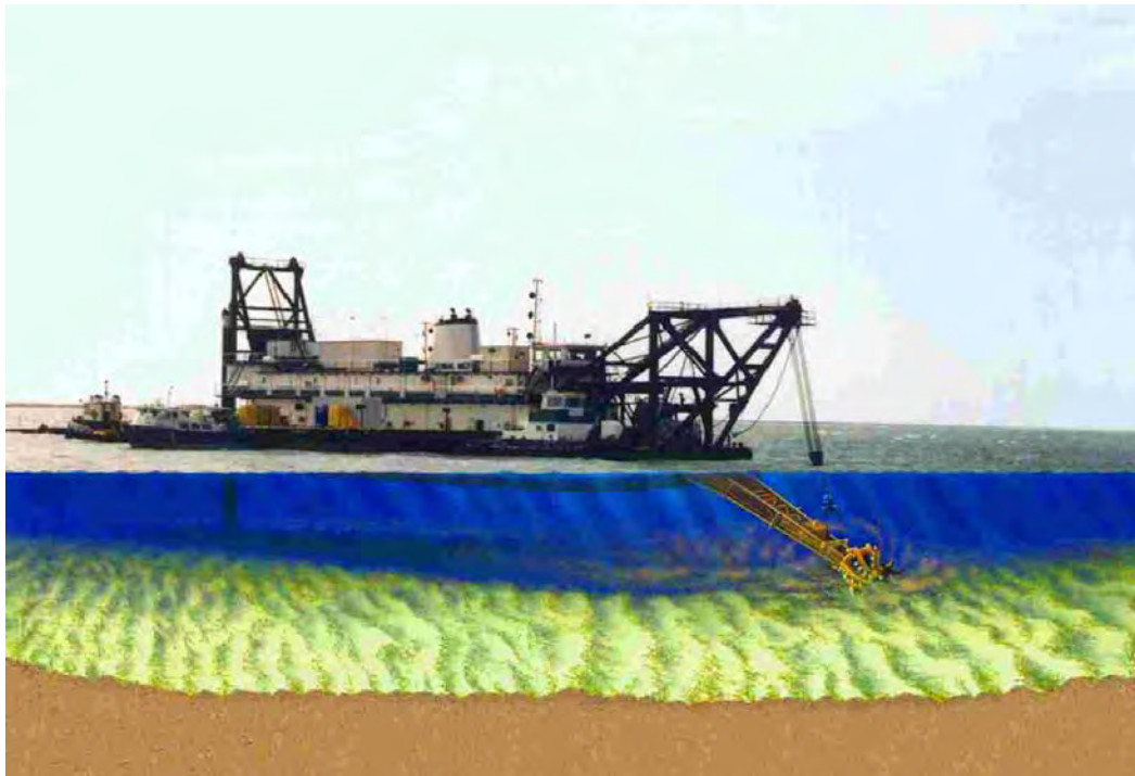
Figure 4. Hydraulic pipeline cutterhead dredge.
