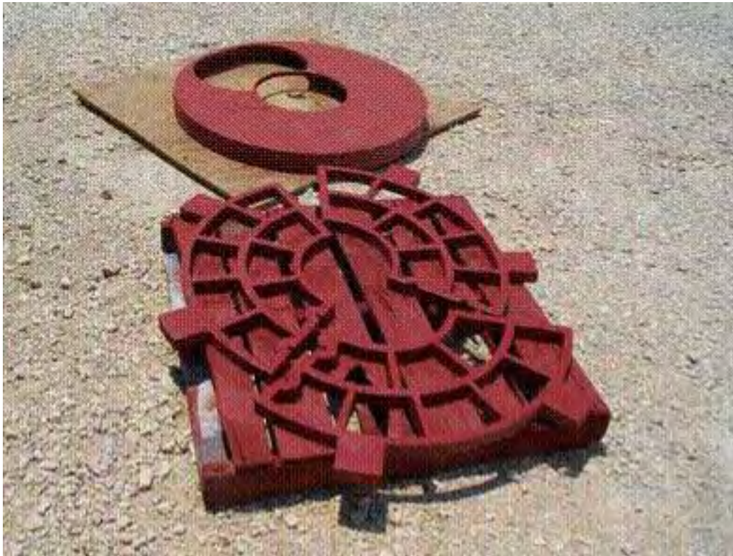
Figure 57. Gatling Gun suction screen (source: DSC).
