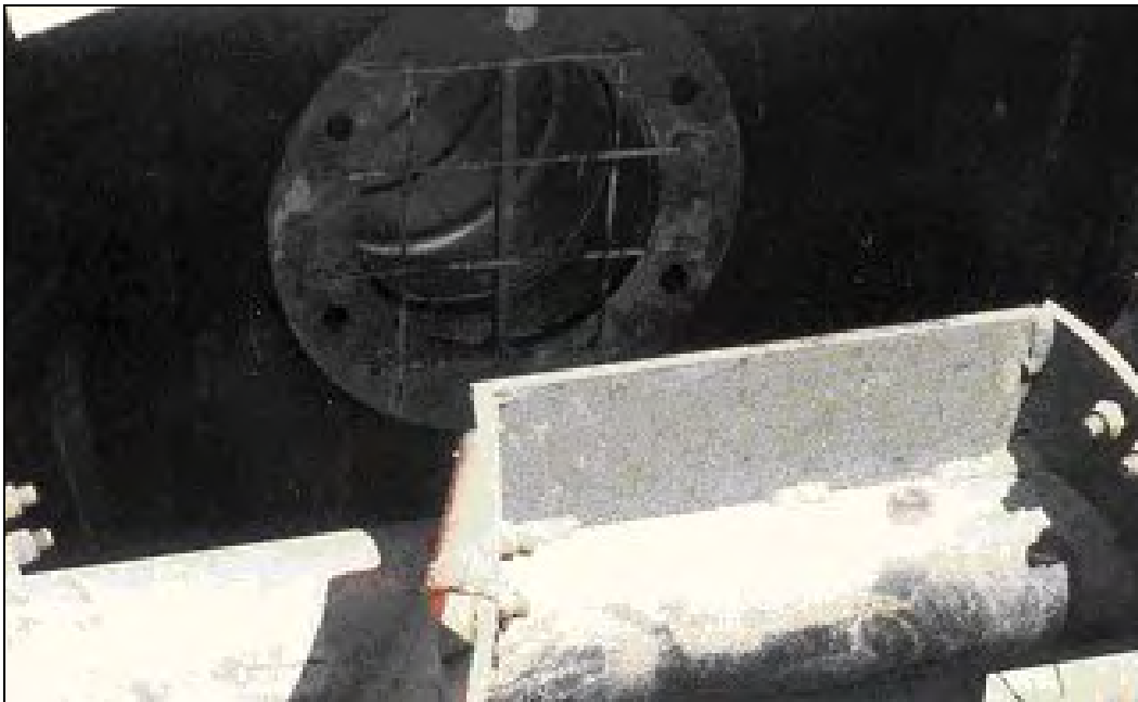
Figure 67. Screen over auger-head suction mouth.
