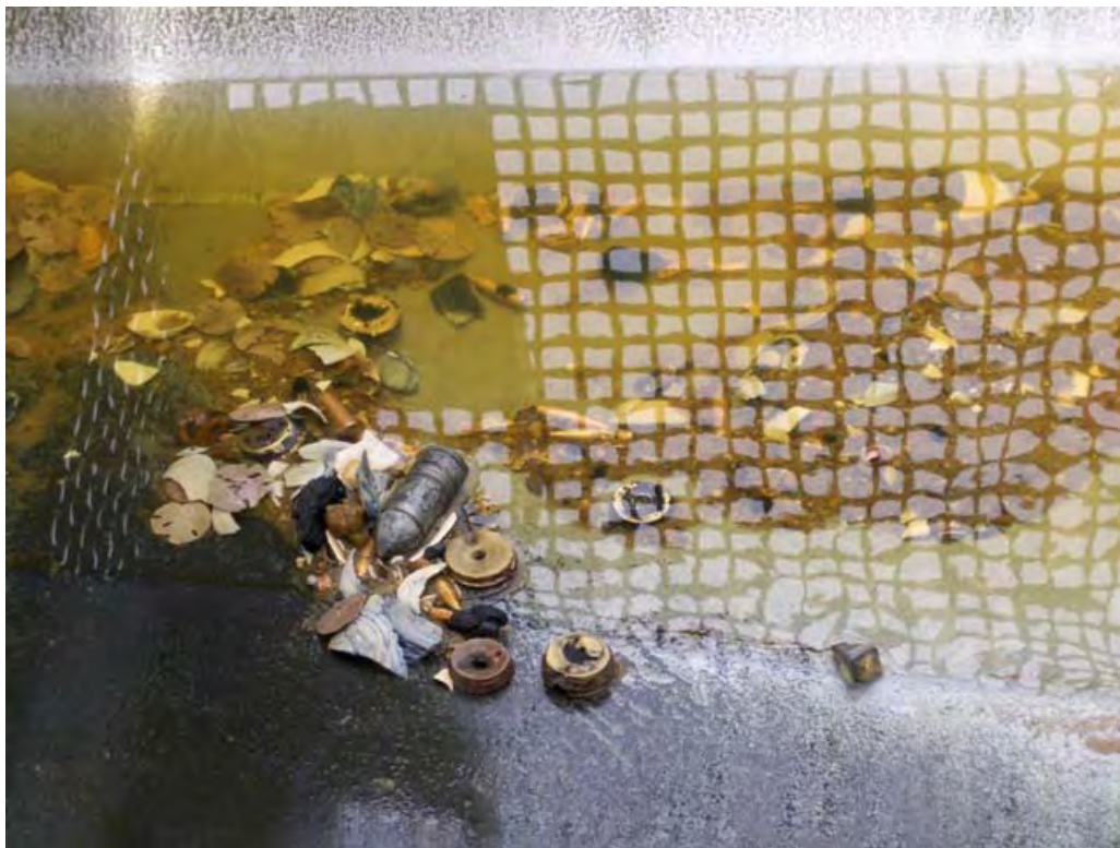
Figure 40. 37 mm armor piercing projectile captured in beach screening basket at Bethany Beach, DE (2007). Note various fuze pieces and .50 caliber projectiles and casings.
