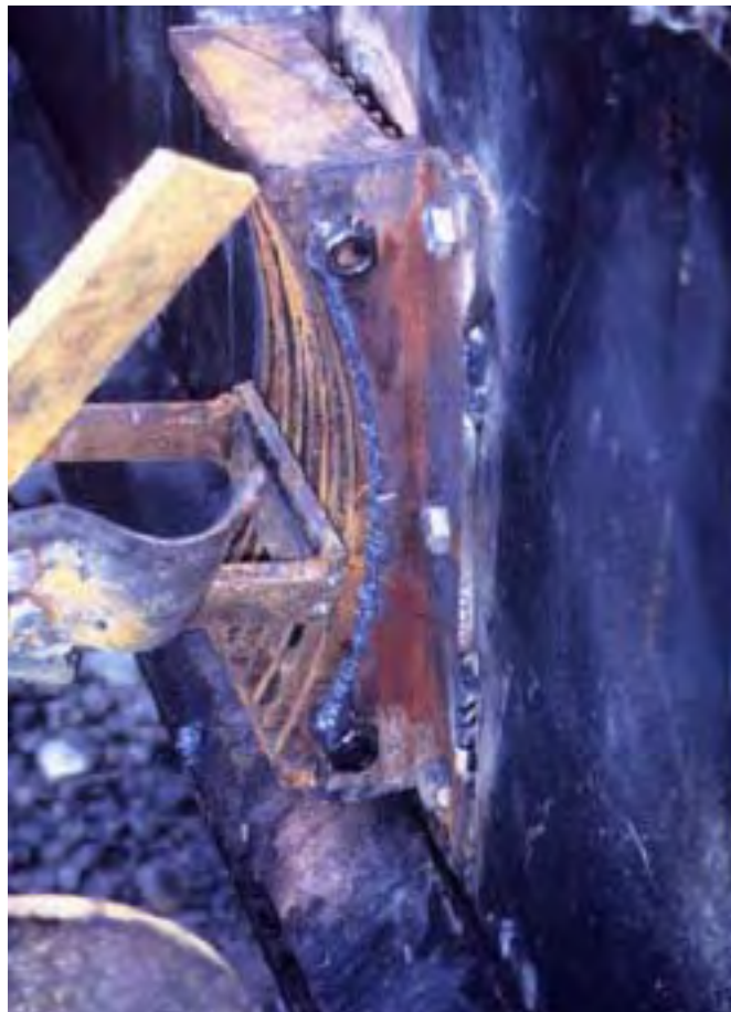
Figure 70. Side view of augerhead suction mouth screen/cutter device (source: Walsh and Collins 1998).
