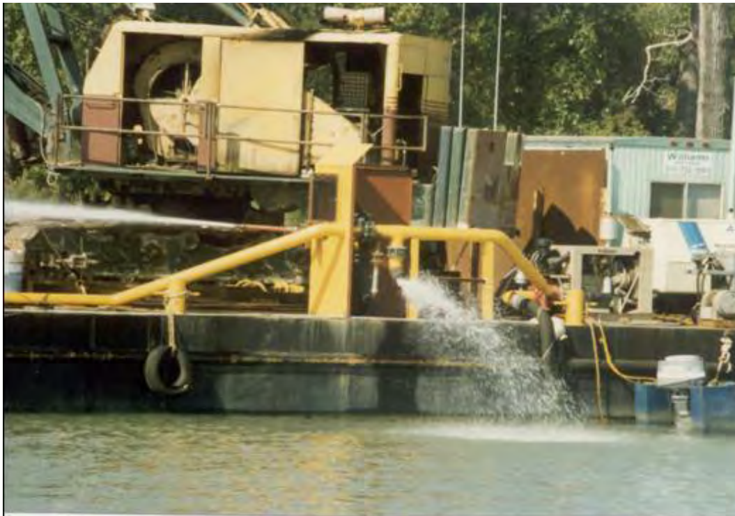
Figure 100. Fluidization valve-control system.
