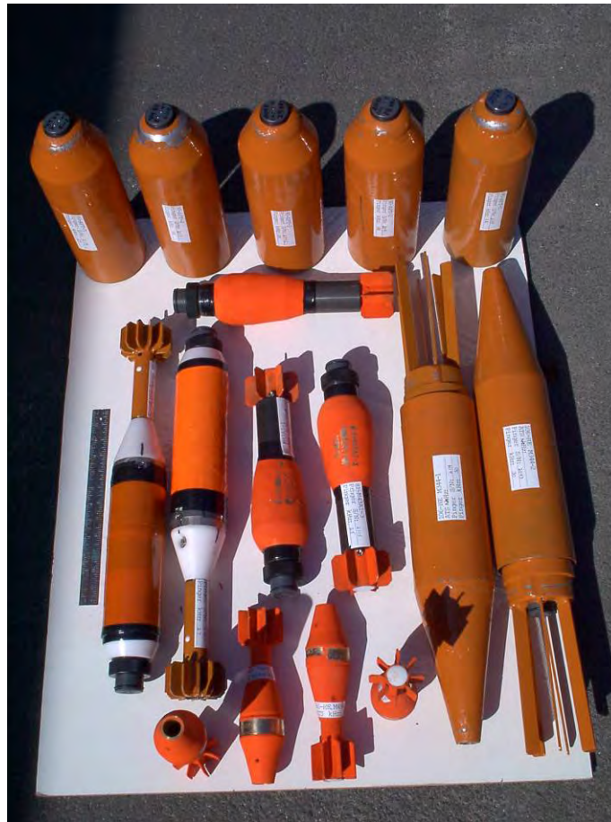
Figure 33. Study sMEC, 16 of 24 sMEC without radio transmitters installed (source: Welp et al. 2004).
