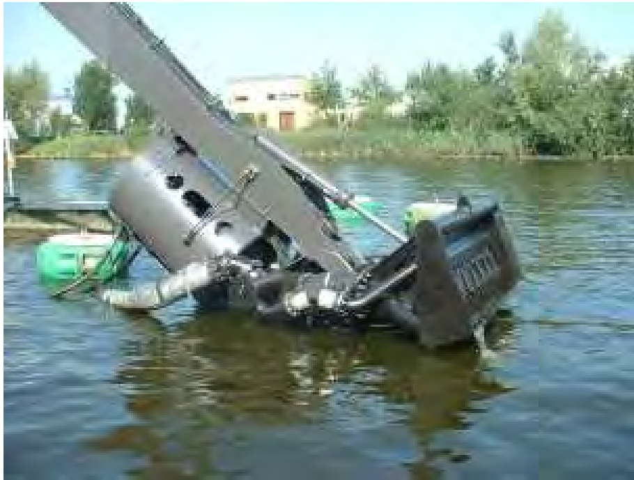
Figure 22. Submersible pump with MEC-exclusion screen (courtesy of Damen Dredging Equipment, The Netherlands).
