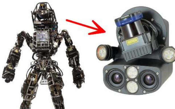
Fig. 1. The Atlas robot contains 28 hydraulically actuated joints, and its primary sensing is provided by the Carnegie Robotics Multisense SL sensor head which is equipped with a rotating LIDAR scanner and a stereo camera. (photo credits: Boston Dynamics and CRL)
