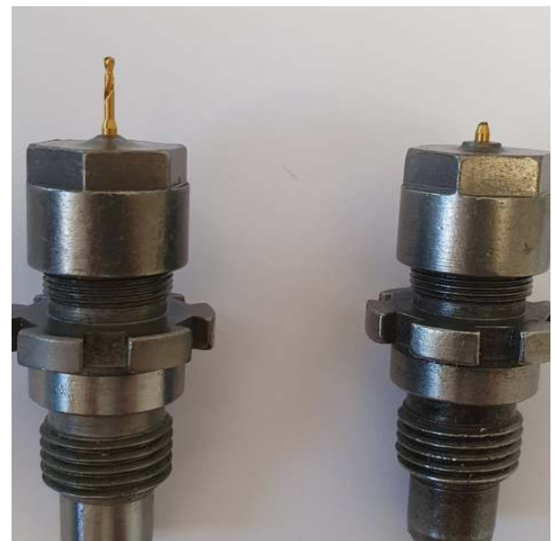
FIGURE 2: A healthy drill bit (on the left side) and a broken drill bit (on the right side).
