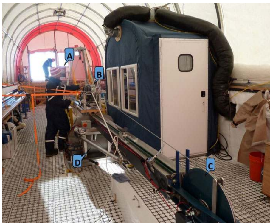
Fig. 17. Spooling and tensioning a new drill cable onto the IDD winch. (a) Spool of new cable. (b) Cable tensioner mounted on the drill tower. (c) The load cell and encoder on the top sheave are used to monitor tension and measure cable length as it is spooled onto the (d) winch spool.
