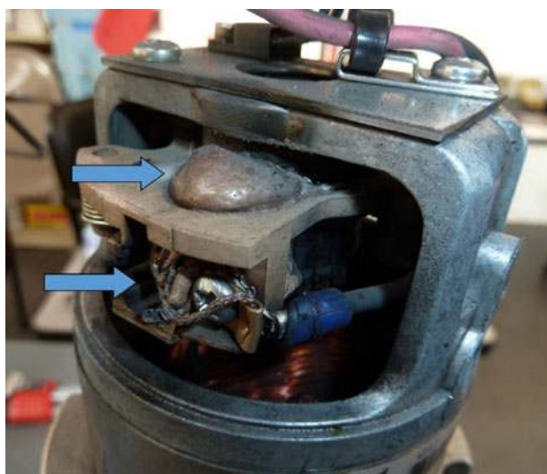
Fig. 16. Drill motor. Arrows point to areas where the brush holder overheated and melted.
