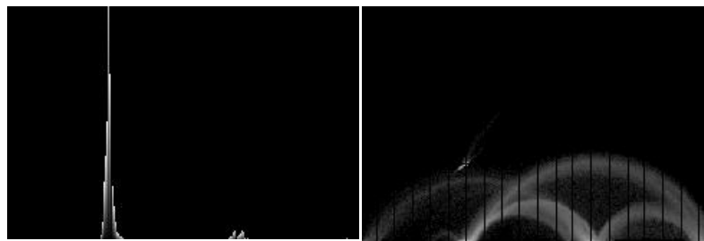
Figure 2. On the left is an value (1D) histogram and on the right is the value-gradient magnitude (2D) histogram of tooth dataset [25]. In both the graphs, value is plotted along the horizontal axis. The gradient magnitude is along the vertical axis in the 2D histogram.
