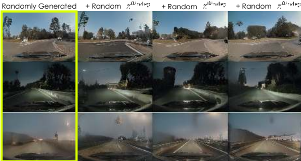
Figure 12: Swapping z^{indep} modifies objects in a scene while keeping layout, such as the shape of the road, consistent. Top: right turn, Middle: road for slight left, Bottom: straight road.
