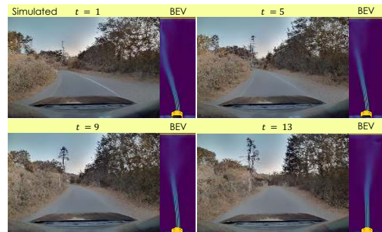
Figure 16: Bird’s-Eye-View (BEV) lane prediction with LiftSplat [40] model on generated scenes.
