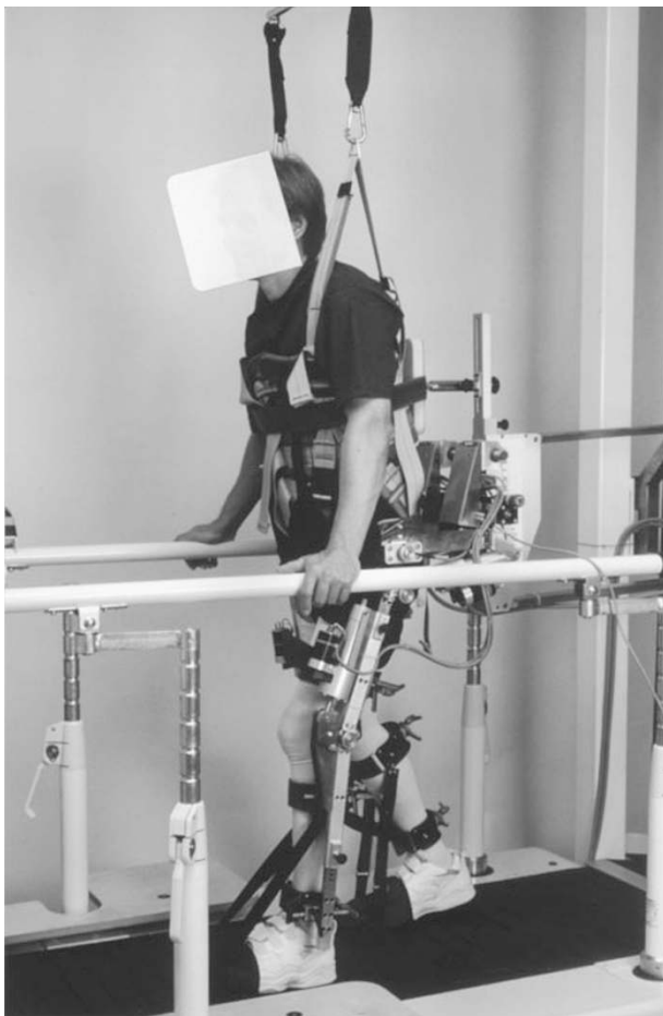
Figure 1 Illustration of a patient with incomplete paraplegia during an automated locomotor training with the DGO
