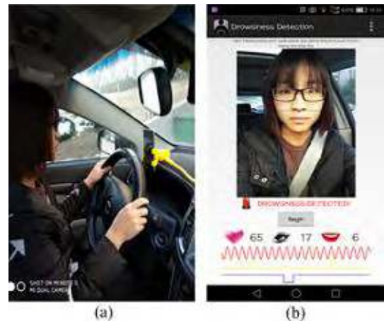
FIGURE 16. The demo runs on a smart phone. (a) The in-car environment for system testing. (b) Screenshot of the system.
